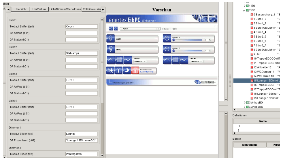
Picture 31: Connecting group addresses with elements
